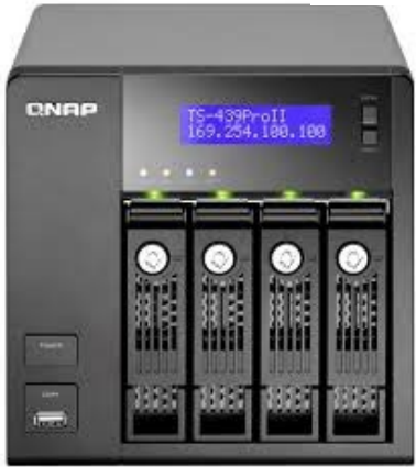
Network Attached Storage (NAS) is a network attached external disk array with multiple hard drives
